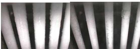
Fig. 10 Frost scattering by jet impingement. Left: before jet impingement, Right: after jet impingement
