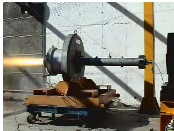
Fig. 7 The Combustion Test of the Pyrogen Igniter with an Inert Chamber
