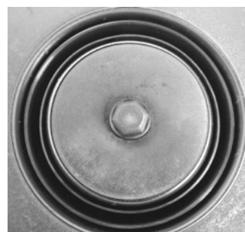
Fig. 2 A hollow anode and an acceleration channel
