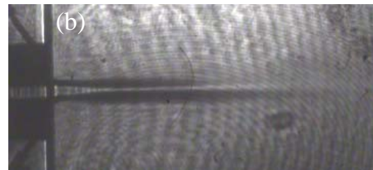
Fig.15 Schlieren Picture ( P=0.20\text{MPa} , P_m=0.51\text{MPa} , (a): w/o microjet, (b): with microjet)
