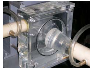
Fig. 3 Centrifugal pump with clear casing and clear impeller
