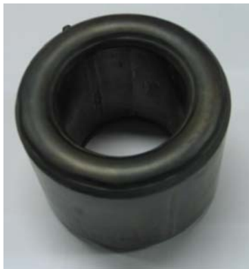
Fig.10 Titanium hollow cylinder tank manufactured by superplastic forming in subscale
