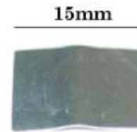
Fig. 6. The plastically deformed aluminum foil due to shock wave unloading.
