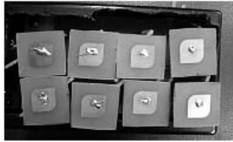
Fig. 5. The picture of eight-rectenna array. Rectifier circuit attached perpendicular to the patch on its back side to minimize antenna pitch.
