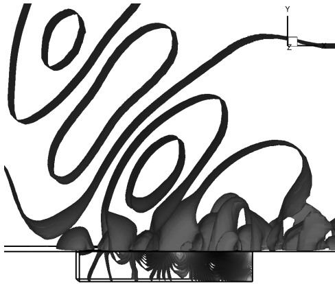
Fig. 2 3-D Acoustic fields of entire domain(M=0.53, L/D=5.5, Re=1.6*10 6 )
