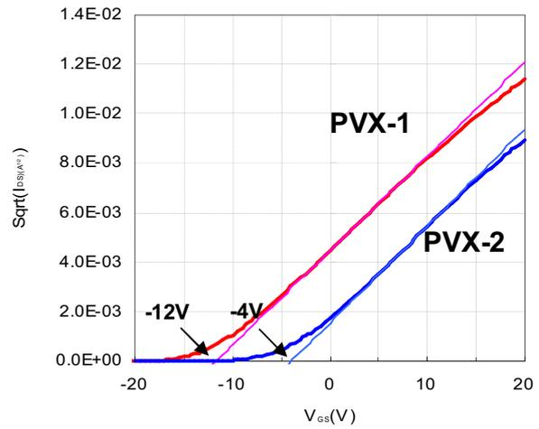
**Fig.5.** Representative threshold voltages of IGZO TFTs according to SiO<sub>x</sub> passivation process conditions (PVX-1, PVX-2) in which the same post-annealing condition was applied
