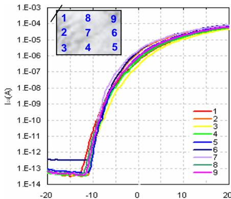
**Figure 4.** Transfer curves of IGZO (700Å) TFTs at 9 positions over a glass: V<sub>ds</sub>=10V, W/L= 25/4μm, with SiO<sub>x</sub> passivation where S/D was wet etched.
