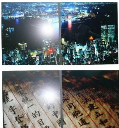
Fig. 4. Comparison of display images on the S-IPS LCD using (a) AG + normal polarizer and (b)ARC+retardation polarizers under the bright illumination intensity at 8,000 lux.
