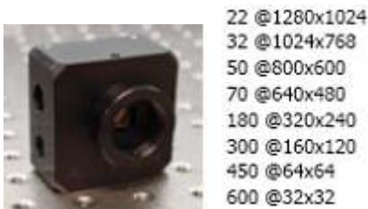
Fig. 1 Camera & Frame Rates
