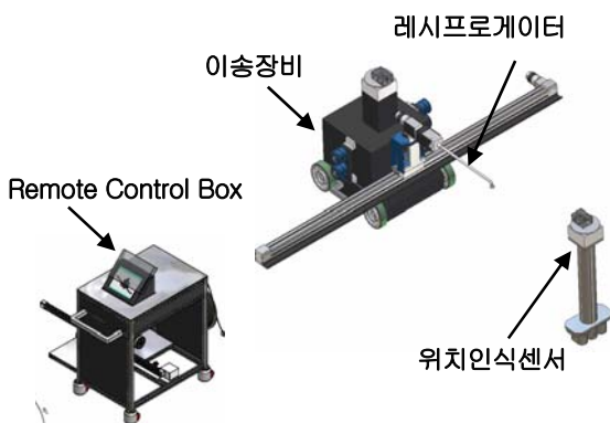
Fig. 1 Developed painting automation equipment
