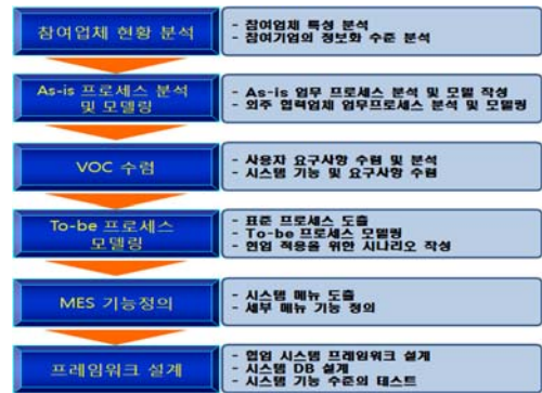
Fig. 1 Design procedure of collaborative manufacturing execution system
