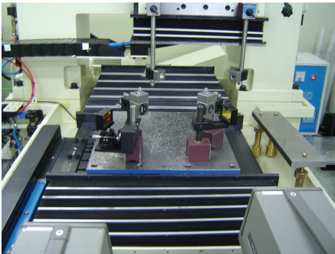
Fig. 3 Positioning accuracy of the X and Y axes
