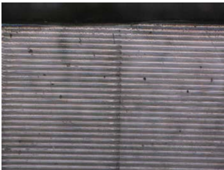
(c) Pattern with stitching error caused by deformation of the PC film
