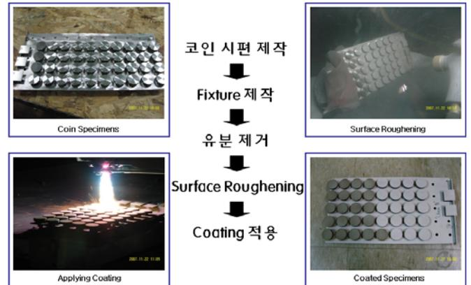
Fig. 2 Coating procedure
