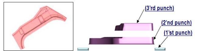
Fig. 3 punch separation
