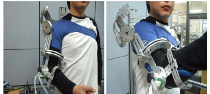
Fig 3. Axis intersection mechanism of shoulder part
