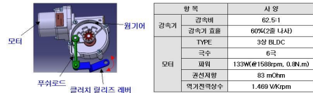
Fig. 3 Clutch actuator model and spec.
