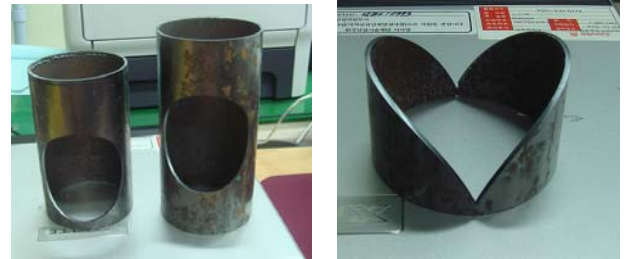
(b) laser cut pipes
