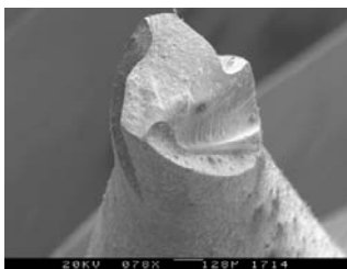
Fig. 2 SEM image of broken micro-end mill
