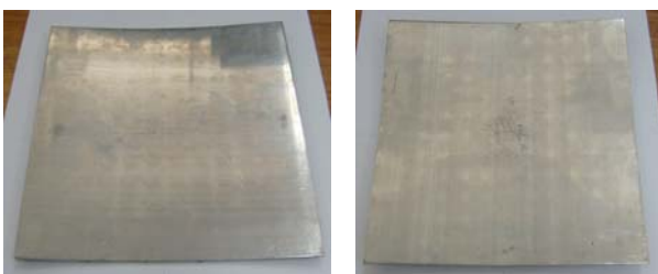
(a) simply curved plate (b) spherically curved plate Fig. 6 Deformed plates through flexible forming process
