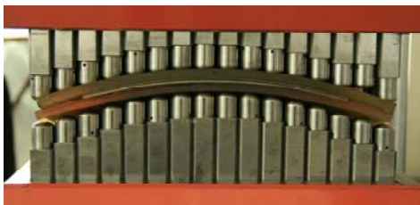
Fig. 5 Plate forming test using flexible press forming apparatus
