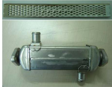
Fig. 2 Dimpled tube and EGR Cooler
