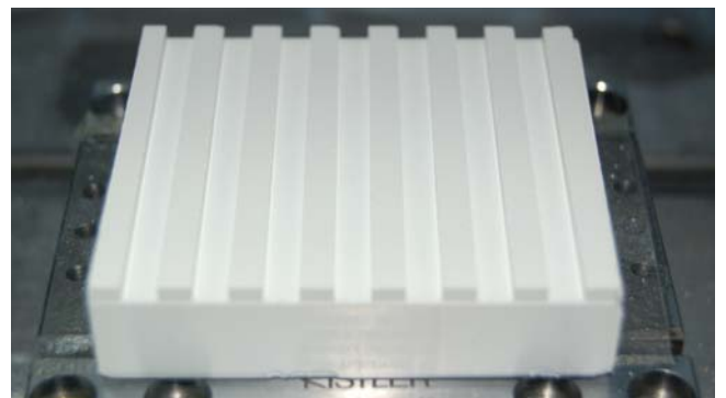
Fig. 2 A workpiece of zirconia for machining experiment
