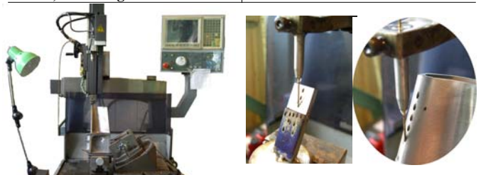
Fig. 1 EDM super drilling machine Fig. 2 Drilling test on flat specimen and cooling hole drilling test
