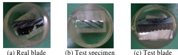
Fig. 3 Cooling hole specimen
