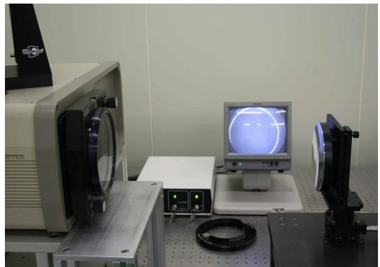
Fig. 6 G-tilt Calibration using Interferometer
