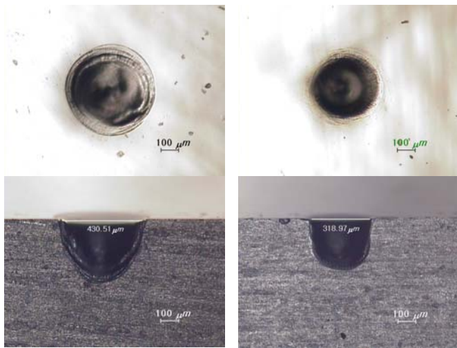
Fig. 2 Cross-section of machined hole using (a) conventional and (b) side insulated electrode at 35 DC rectified voltage and 20 wt % NaOH solution
