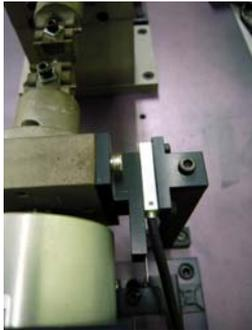
Fig.5 Strain measurement at displacement sensor (linear scale sensor)
