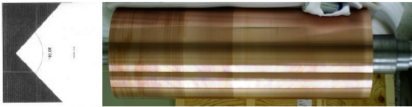
Fig. 3 Single Crystal Diamond Tool & Roll Mold
