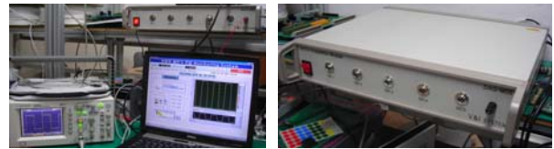
Fig. 6 Monitoring system to measure the voltage
