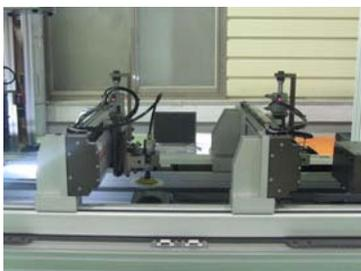
Fig. 6 Structure of polishing process using 2-Axis robot
