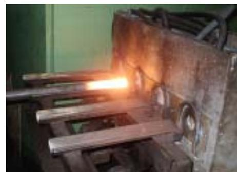
Fig. 4 Output of heating billet
