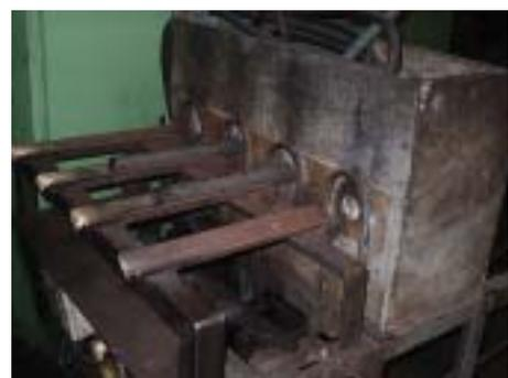
Fig. 3 Billet heating machine
