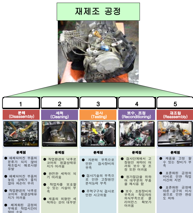
Fig. 1 Detail process of remanufacturing
