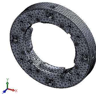
Fig. 5 Finite element model of the auto clamp device
