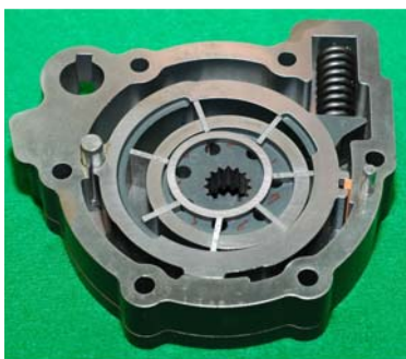
Fig. 6. Assembly of prototype vane pump
