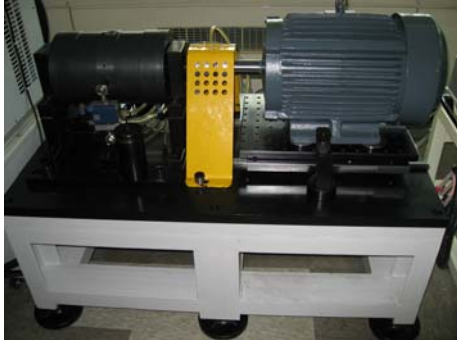
Fig. 2 Dynamometer connect to the induction Motor
