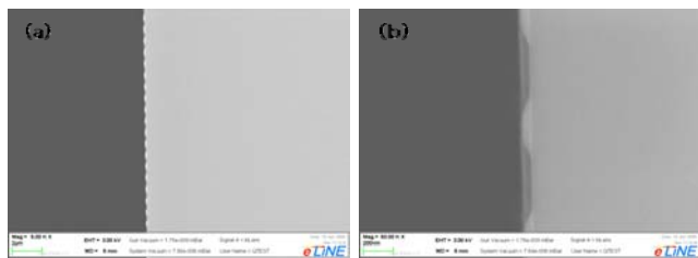
Fig. 4 SEM images of the cross sectional silver patterns by nanoimprint lithography using a PDMS stamp with Xylene (a) x50000 (b) x50000.
