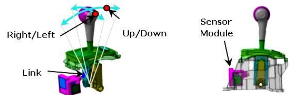
Fig. 2 Structure of Lever CAN Module
