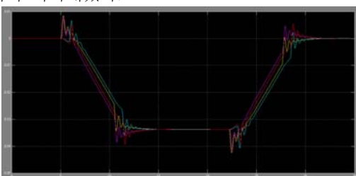
Fig. 4 Yaw angle of leading & trailing wheelsets of each bogie for active steering railway vehicle
