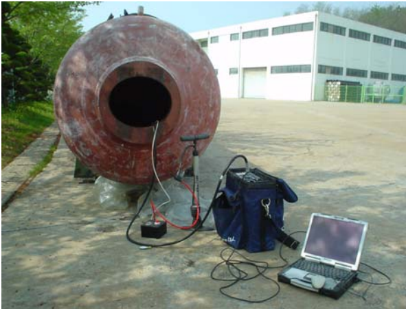
Fig. 2 Field test for U-Type feedwater heater
