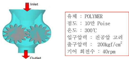
Fig. 6 Model of flow rate analysis
