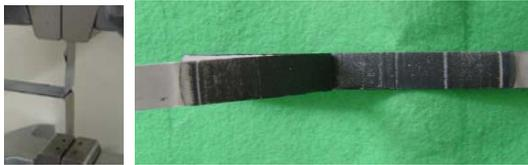
Fig. 5 T-peel test specimen and its cohesive failure mode
