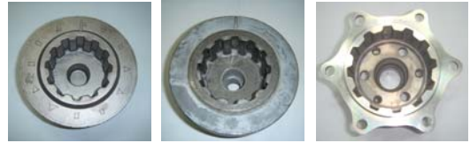
(a)Hot forging (b) Cold forging (c) Final part Fig. 2 Diff. case of cam type for 4WD auto bicycle
