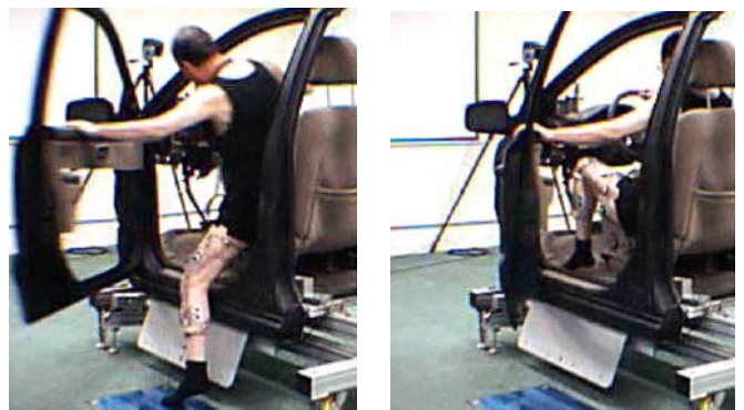
Fig. 1 Ingress movement at a 1/4 unit mockup
