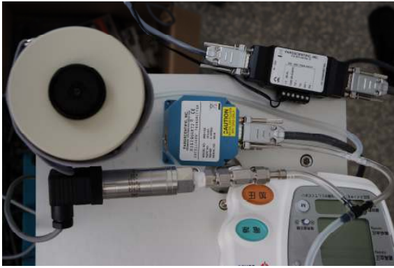
Fig. 3. Experimental arrangement for the check of measurement repeatability
