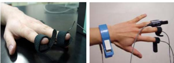
Fig. 1 Electrode of GSR & HR
