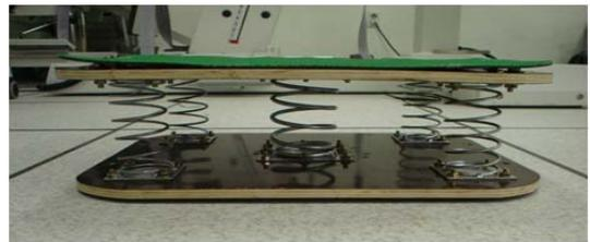
Fig. 2 Unstable platform with stiffness spring
