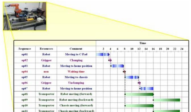
Fig. 3 Sequence diagram based on process analysis
