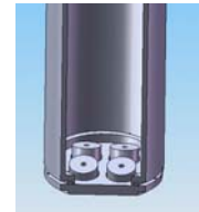
Fig. 5 4 Column Electron Beam Column Array Concept
